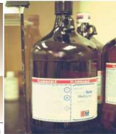
Figure 25-35 This glass jar is coated with a plastic coating that will not allow the liquid to spill out if the glass is broken or dropped.
