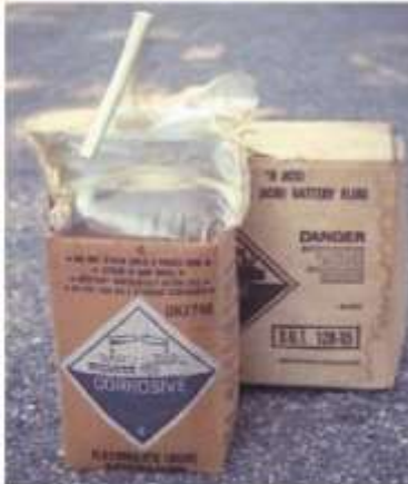
Figure 25-33 Typically, chemicals that can cause harm are not packaged in cardboard. This sulfuric acid is one example of a material that can cause harm, but unfortunately is packaged in cardboard.
