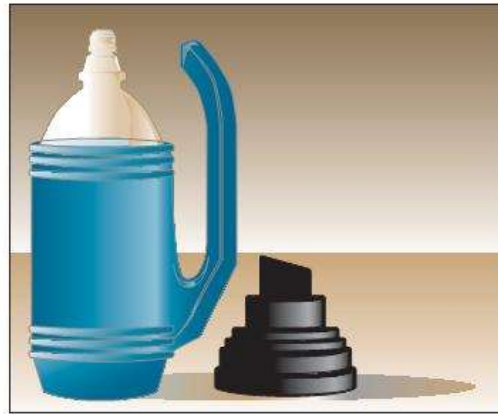
Figure 25-34 To protect the glass bottle, which has a corrosive in it, a carboy is used in case the bottle is dropped.
